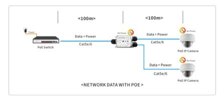
Diagram 2. UPoE+ Extender provides enough power to allow 300 metres (984 ft) of extension to a POE Plus wireless access point, using two UPoE+ Extender units located at 100 metre intervals.
